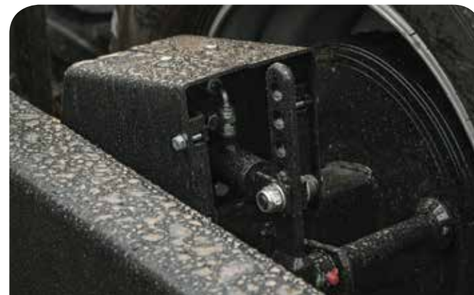
Hydraulic and pneumatic brake options with protections.
