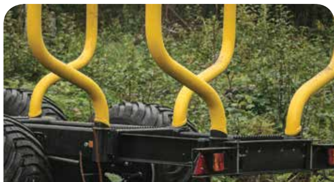
Frame extension to maximize the loading length.
