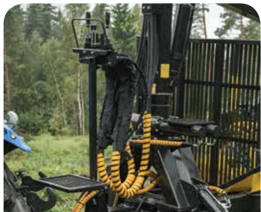
Stative for operating the valve block from outside platform.
